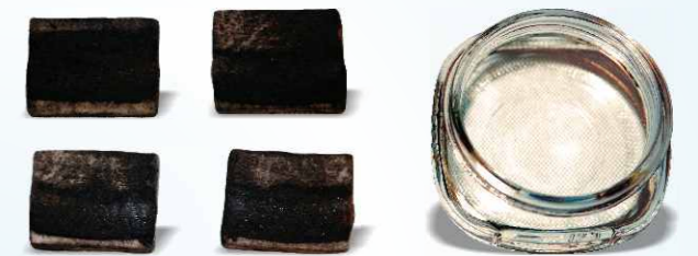
Fig. 1: Felt pads from slitter & scorer before treatment with Turmocut SR 15
